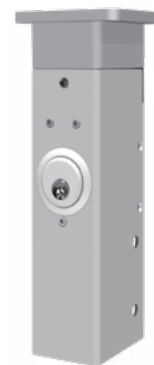
KR90F 694.00 Standard Key Removable Mullion Less Key Cylinder For Panic Exit and Fire Exit Rim Mount Devices. Length: 8ft Material: 2" 11 Gauge Steel Tube Finish: Primer gray
